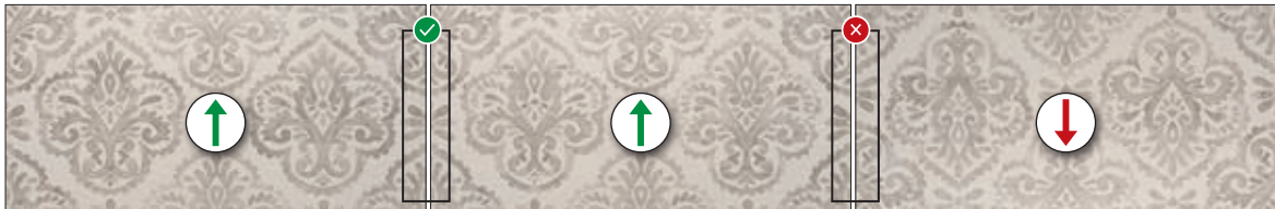
example of correct and incorrect alignment
